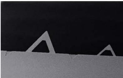
Fig. 1: Pyrex-Nitride oxide sharpened, pyramidal tip
