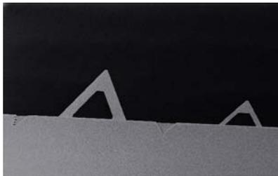
Pyrex-Nitride™ Triangular Tipless Cantilever
